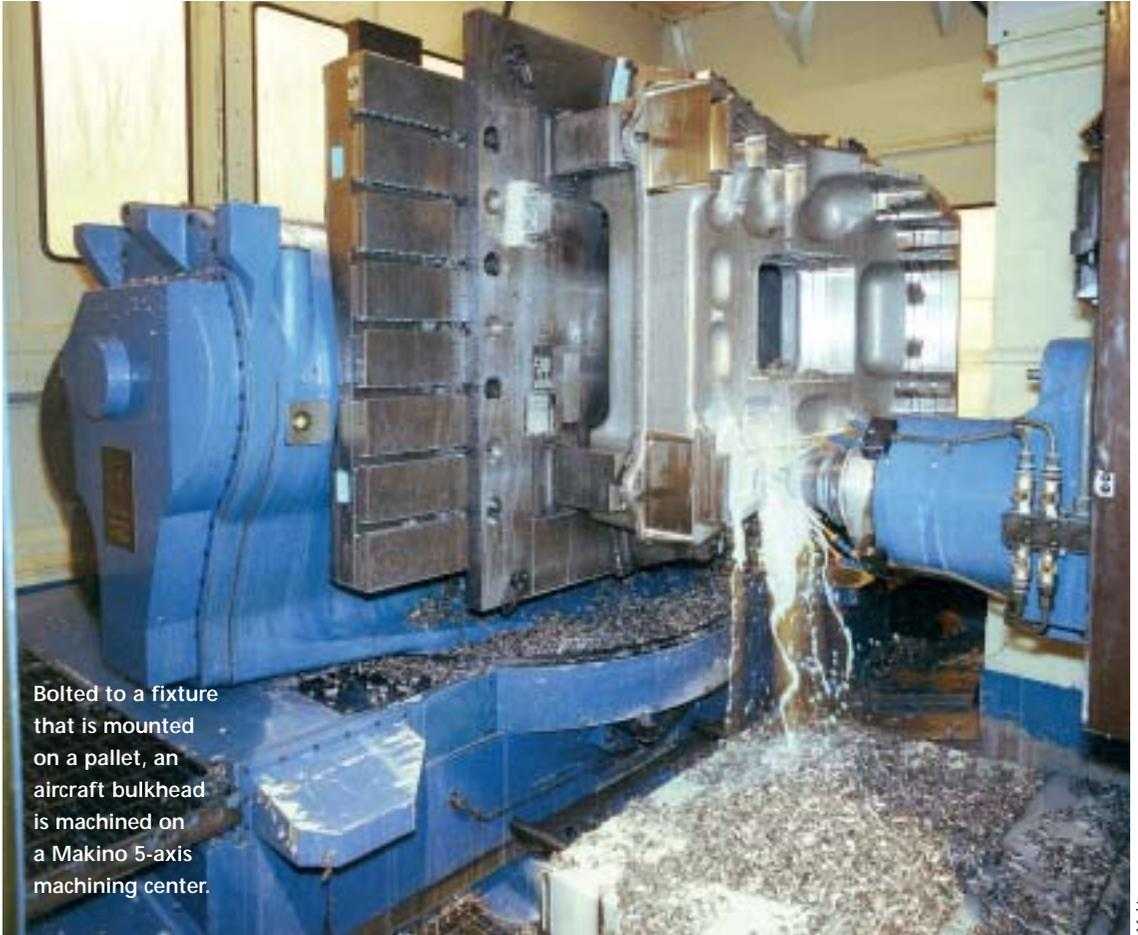
Bolted to a fixture that is mounted on a pallet, an aircraft bulkhead is machined on a Makino 5-axis machining center.
